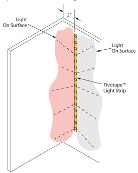
**Note 2:** In applications where multiple strips of Tivotape<sup>TM</sup> are reflecting on a common surface, it is recommended that the tape be mounted at least 2'' away from the reflecting surface and oriented with the same edge of Tivotape<sup>TM</sup> mounted closest to the outside edge, as shown. Note the position of the lead end.
